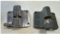
Left: 3D printed replacement part Right: original part damaged in field operations
