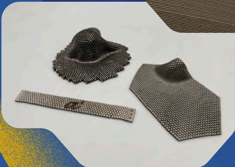
Left: AM Process-Printed parts using A*STAR SIMTech developed micro-LPBF
