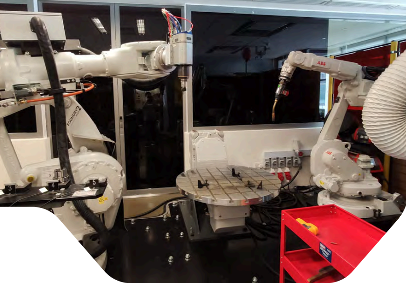
Left: Large Format Printing Platform Solution—Hybrid Wire Arc Additive Manufacturing (WAAM) system at SUTD
