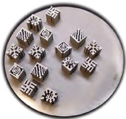
3D Printing Build Plate with Interactions Cubes: Each cube has a side length of 0.98 cm and is made from Inconel, a nickel-based superalloy.
