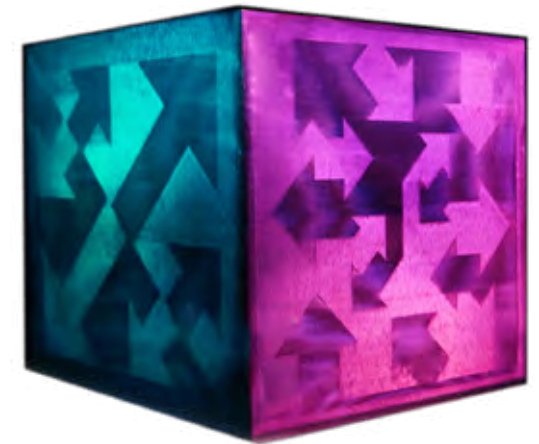
Structure & Reflectance Cube in Stainless Steel (15 cm) Printed Using LPBF Technology: A scaled-up prototype of the two cubes that went to the International Space Station and will soon go to the Moon.
