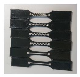
The various geometries of the conductive traces experimented within the scope of this project.
