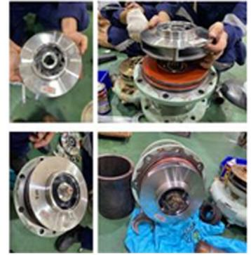
Figure 7: Installation of printed pump impeller
