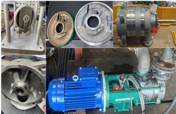
Figure 3: Pump assembly using AM-built parts
