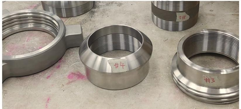
Figure 8: Printed Connectors after NDT Testing
