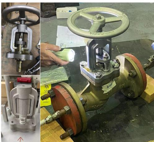
Figure 4: Valve assembly using AM-built parts
