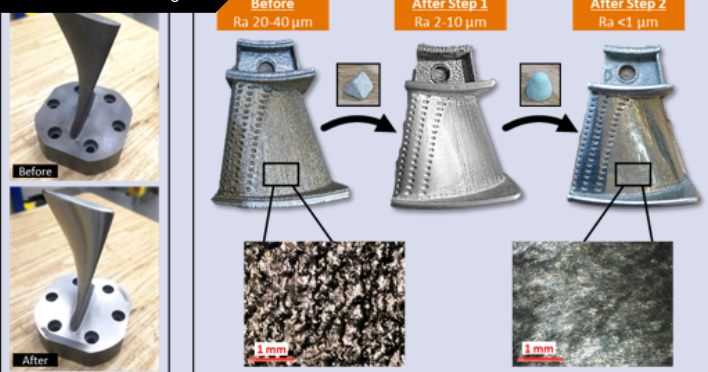
Polishing of L-PBF component
