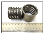
Sectioning by wire-EDM
