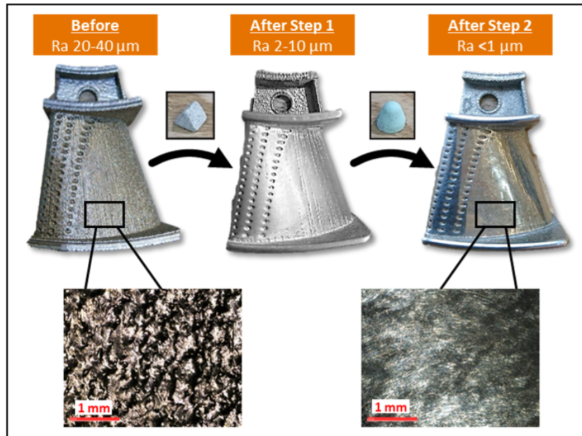
Polishing of EBM component
