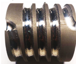
Sectioning by wire-EDM
