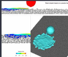
**FLOW-3D** models resin infiltration and lateral spreading in a powder bed during a binder jetting 3D printing process. Fully and accurately resolving the particles and voids within a particle bed enables analysis.
