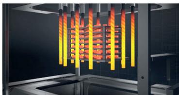
The Production System – sinter process to remove remaining binder and densify the metal particles
