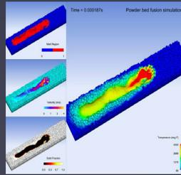
The effect of process parameters (laser power, scan patterns and speed) on underlying physical phenomena (melt pool dynamics, phase change & solidification microstructure evolution, porosity formation in keyhole welding, balling defects & microstructure prediction in L-PBF processes, and crystal growth & orientation in direct energy deposition processes) can be modeled in FLOW-3D.
