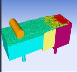
Using the discrete element method, **FLOW-3D** is able to accurately simulate the powder packing and spreading processes. Models to study particle-particle interactions, particle-roller/knife interactions, and full particle-fluid flow coupling for various particle size distributions are available.
