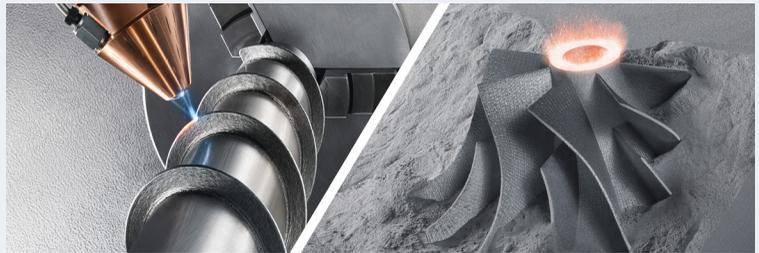
For additive manufacturing, TRUMPF provides you with solutions in both relevant laser technologies: laser metal fusion (LMF) and laser metal deposition (LMD). Depending on the application, we offer the right 3D printer or laser processing machine for your industrial manufacturing processes.
