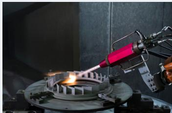
Supercoat by High Velocity Oxygen Fuel (HVOF)
