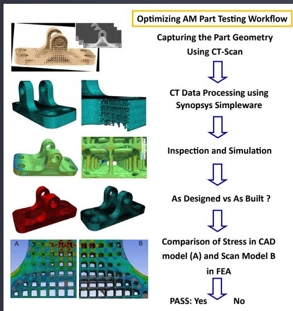
Going from a 3D computed tomography (CT) scan of an AM part to a completed simulation is achieved by using Synopsys Simpleware™ software as a crucial bridging technology that generates high-quality meshes from CT Scans. Results from test workflows show the differences between as-designed and as-manufactured parts, catching unexpected defects early in the design stage and saving on long-term costs caused by manufacturing errors.
