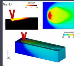
In direct energy deposition processes, process parameters such as powder injection rate, particle size distribution, laser power and scan speed can influence the printed layer thickness and crystal orientation. **FLOW-3D** can simulate the DED processes in fine detail to achieve better process control of multi-layer deposition.
