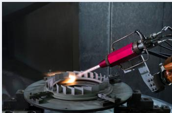
Supercoat by High Velocity Oxygen Fuel (HVOF)
