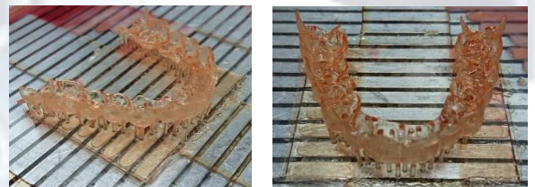
Dental aligners fabricated from the developed SMP
