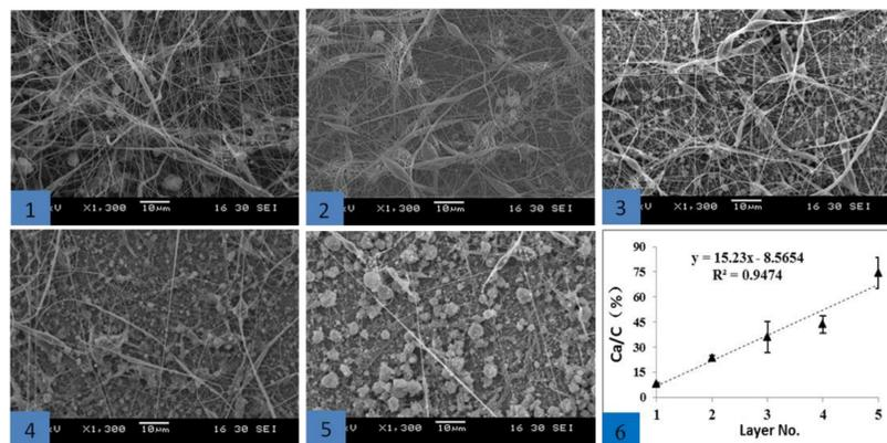
**Figure 2:** (1-5) Morphology of different layers of the scaffold; (6) The C/Ca ratio of different layers of the scaffolds.
