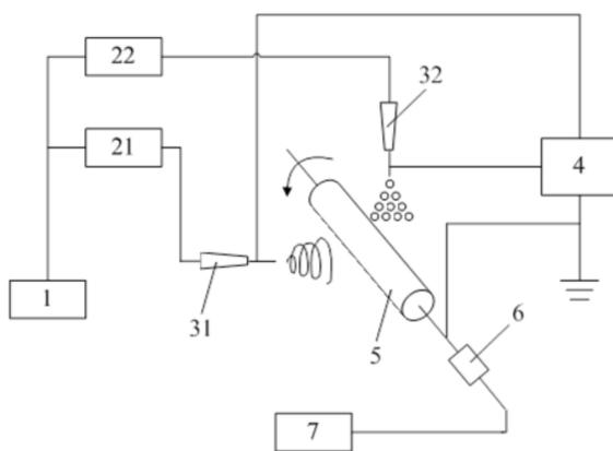
**Figure 1:** Schematic overview of the hybrid E-spinning and E-spraying system.
